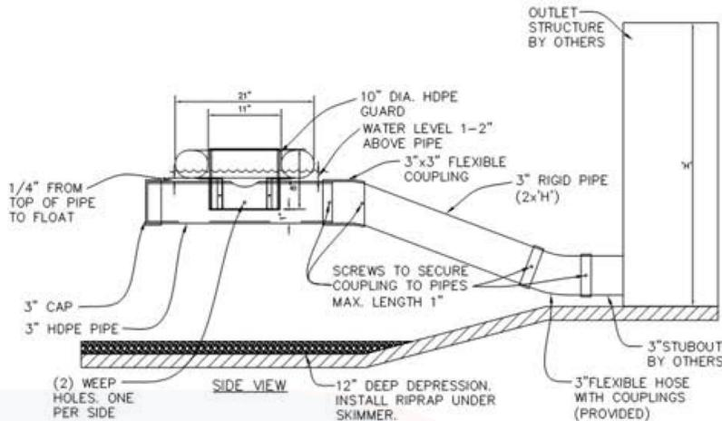
1. Model 1: 1" - 2.5" Marlee Float Skimmer is to be attached to a 3" rigid pipe (Schedule 40 PVC for construction/temporary applications or HDPE for permanent applications). Rigid pipe should be 1.5 times the height of the outlet structure (H), minimum of 6'.
