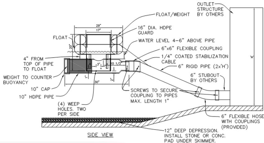
1. Model 3: 5" - 8" Marlee Float Skimmer is to be attached to a 6" rigid pipe (Schedule 40 PVC for construction/temporary applications or HDPE for permanent applications). Rigid pipe should be 1.5 times the height of the outlet structure – minimum of 8'. For ponds requiring a pipe length greater than 14' additional weight may be required to counteract buoyancy.
