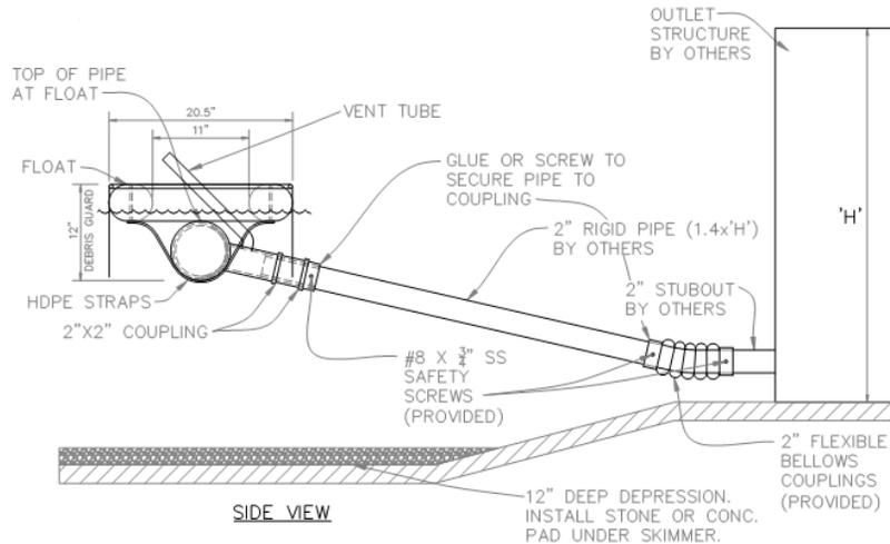
1. 2" Marlee Float™ Skimmer is to be attached to a 2" rigid pipe (Schedule 40 PVC for temporary applications or UV-Resistant PVC or HDPE for permanent applications). Rigid pipe should be 1.4 times the height of the outlet structure – minimum of 8'.
